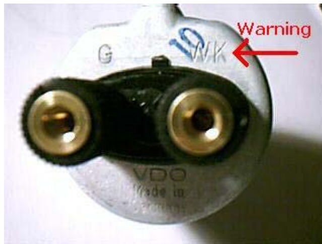
(Figure 9, location of "WK" lead for the grounding of lamp or buzzer)
