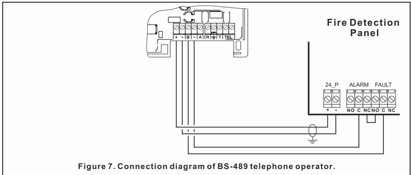
Figure 7. Connection diagram of BS-489 telephone operator.
