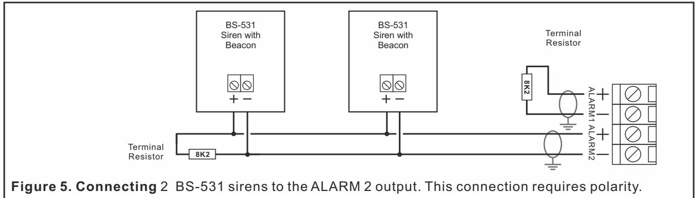
**Figure 5. Connecting 2 BS-531 sirens to the ALARM 2 output. This connection requires polarity.**
