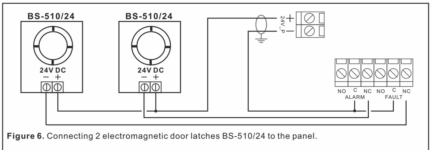
**Figure 6. Connecting 2 electromagnetic door latches BS-510/24 to the panel.**
