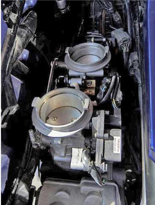
3. Install the DNA DN-9410-R2 NITRILE L-RINGS supplied, on the throttle bodies.
