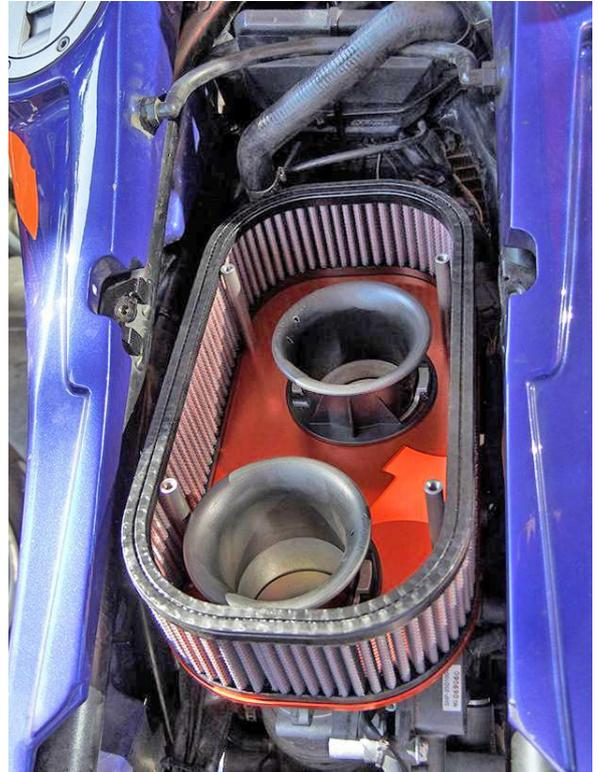
7. Install the top of the DNA S3 Air Box Kit and bolt it in place (MK3 is displayed below left & MK1 is below right)
