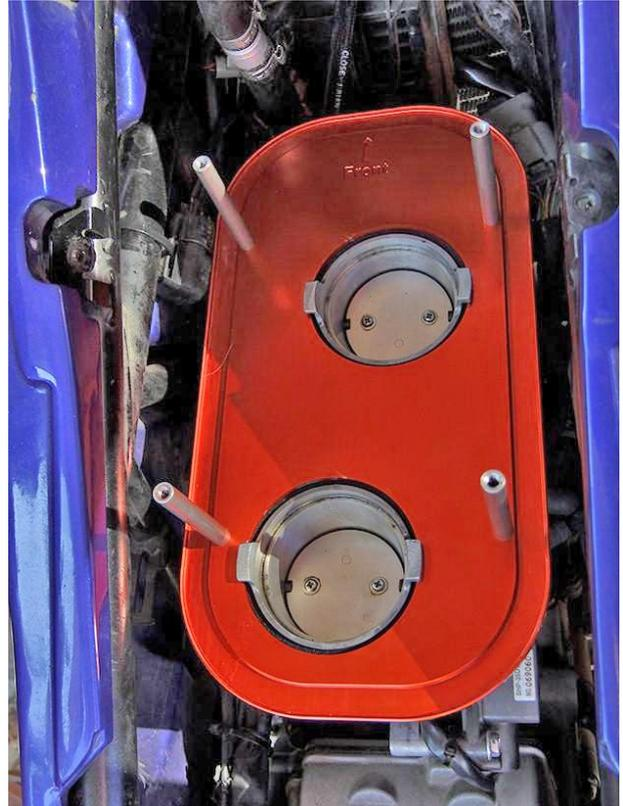
5. Install the velocity stacks in place, rotating them 45 deg. to lock.
